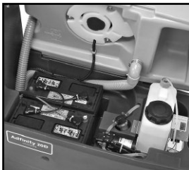
Access to batteries and AXP onboard dispensing system
