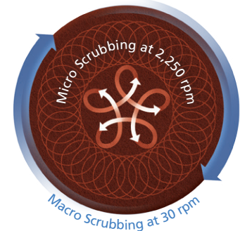
Patented REV random orbital scrubbing technology with high-speed, ¼-inch micro scrubbing and rotational, low-speed macro scrubbing attacks dirt from multiple directions for superior cleaning effectiveness.
