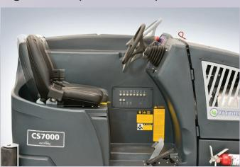
The CS7000 has a fully adjustable seat and tilt steering.
