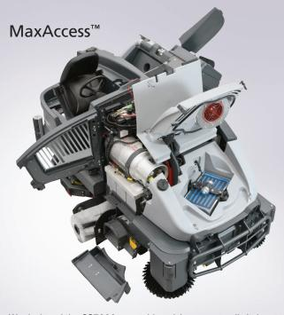
We designed the CS7000 to provide quick access to all vital systems for easier inspection and maintenance.
