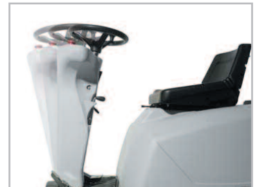
Adjustable steering column and seat provide comfort and easy accessibility to enter and exit the operator's position.
