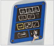
True One-Touch™ operation. Press a single button to lower the squeegee and activate the system.
