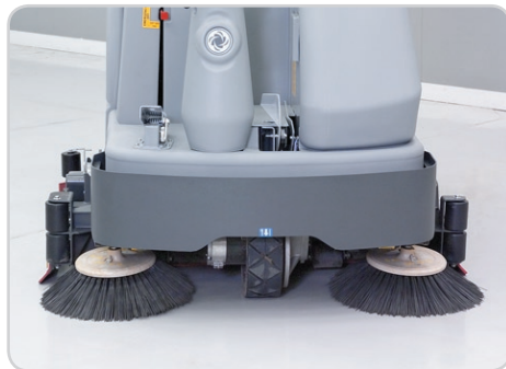
Retractable side brooms on cylindrical models sweep debris away from pallets and walls.
