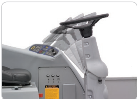
Ergonomic command compartment with tilt steering allows for easy ingress and egress.
