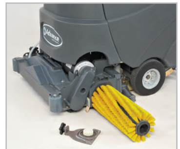
Tools-free removable brushes make for easy clean-up after use
