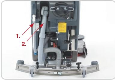
1. Solution level indicator also functions as solution drain hose
