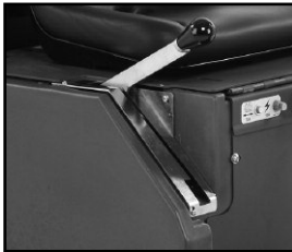
Mechanical deck lift lever
