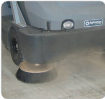
DustGuard™ suppresses side broom generated dust increasing dust controlled productivity by up to 71%.
