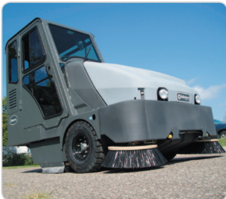
The optional all weather cab keeps the operator comfortable and productive. Clear-View™ window in the cab provides a safe view of the right side broom.
