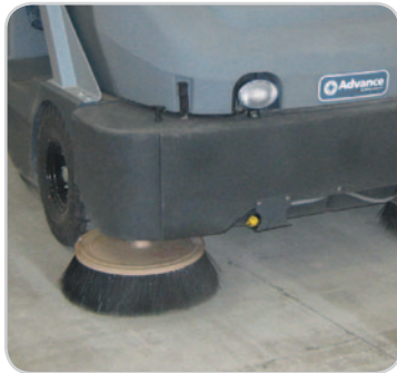
DustGuard™ suppresses side broom generated dust increasing dust controlled productivity by up to 71%.
