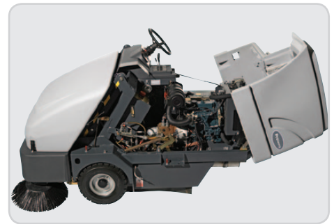
MaxAccess™ allows faster repairs and less downtime so the sweeper spends less time in the shop and more time sweeping
