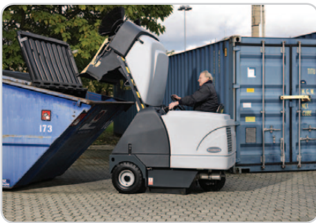
Variable dump height of up to 62 inches allows fast and simple disposal of swept debris
