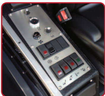
Infinitely variable water pressure and cleaning speed is easily controlled from the operator's seat, for a full clean on various surfaces.
