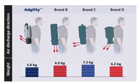
an angle are more comfortable for the operator but may have a tendency to disturb nearby surface dust or papers on desks. Units that direct the hot-air discharge away from the operator and upward have been judged to offer the most comfort and also to be less likely to disturb papers or surface dust.
