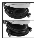
The SC351's rotating deck allows for both forward and backward scrubbing. Operators can push the machine forward in all directions like a "normal" scrubber. But, if the application requires, operators can quickly flip the machine up, triggering the deck to rotate completely for backward scrubbing performance. The scrub deck efficiently guides the wheels for superior edge cleaning.
