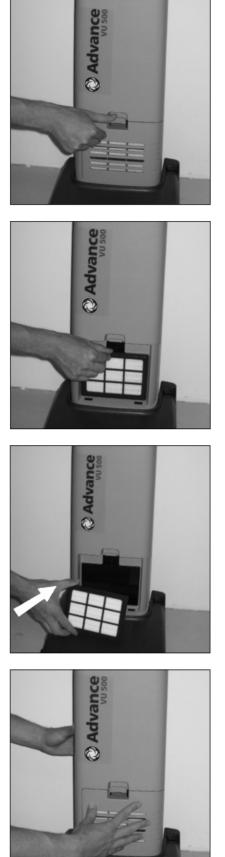
Disconnect the power cord from the electrical outlet. Push the Filter Cover Latch (13) downwards so that the cover is released. Remove the filter cover from cleaner.
