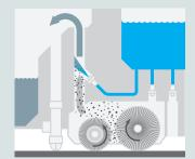
**Dry Sweep Mode** with dual brushes for daily sweeping and two-stage filtration for complete dust containment
