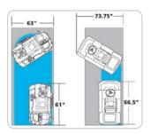
The Adgressor® turns within a 63 inch (160 cm) aisle. This improves productivity by allowing the Adgressor to easily clean smaller aisles than the competition.
