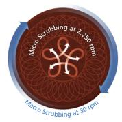
REV model only – Patented REV™ random orbital scrubbing technology with high-speed, ¼-inch micro scrubbing and rotational, low-speed macro scrubbing attacks dirt from multiple directions for superior cleaning effectiveness.
