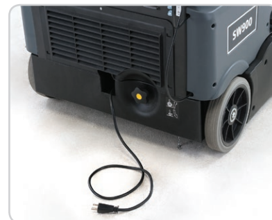
An onboard charger provides the convenience of charging anywhere a power outlet is available.
