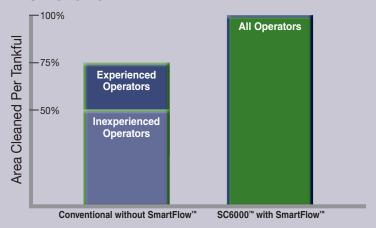
SmartFlow™ adjusts solution flow with the machine's speed, using up to 50% less water and chemicals. Proportionally higher productivity with fewer dump and refill cycles per tankful.
