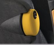
Conveniently located thumb controlled cruise control increases productivity and safety.
