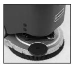
Adjustable machine deck provides increased down pressure to optimize scrubbing for heavy-duty applications.
