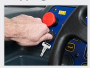
**1** To stop the machine, turn the CS7000 ignition key **OFF**.
