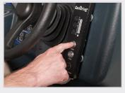
**1** Turn the fuel cell on by pushing the **START** button.
