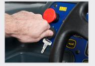
**2** Turn the CS7000 on by turning the ignition key **ON**.
