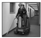
A standard detailing wand offers the ability to clean base boards without leaving the operator compartment.
