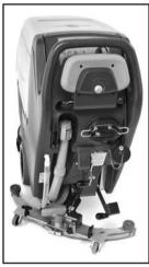
Easy access rear-port features include the solution tank fill, a large recovery drain hose with pinch-flow regulation, and the solution drain hose which also functions as a solution level indicator.
