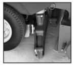
Dual laminar flow vac shoes allow for more efficient recovery of solution.
