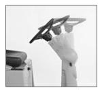
Steering is adjustable to five positions for operator comfort.
