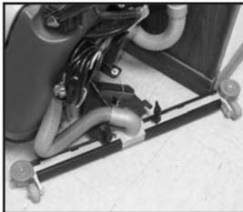
“Break-away” rear squeegee prevents damage to machine and facility.
