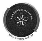
REV<sup>™</sup> model only – Patent-pending REV<sup>™</sup> random orbital scrubbing technology with high-speed, ¼-inch micro scrubbing and rotational, low-speed macro scrubbing attacks dirt from multiple directions for superior cleaning effectiveness.
