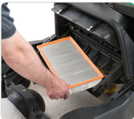
Single-stage high capacity dust control system for more effective dust control. Access filter without tools.
