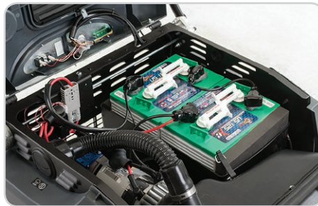
Hood opens providing full maintenance and service accessibility to the battery compartment.
