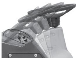
Clear-View™ design and adjustable tilt steering column enable an ergonomic ride for most operators.
