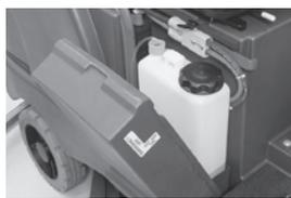
Removable, high capacity detergent cartridge for sustained flexible cleaning is available with optional EcoFlex™ System.
