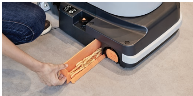
Easily access the debris tray to empty and clean.
