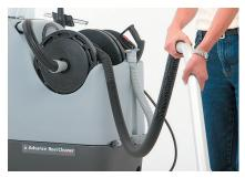
The 40-foot recovery hose is a 5:1 stretch hose for a minimum amount of hose to manage.
