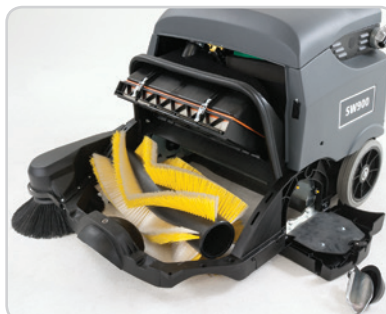
Time-saving maintenance: Broom replacement, and other routine maintenance, can be performed without tools.
