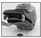
Pad changes are easier with the tip back design of the BU800<sup>™</sup>.
