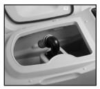
Large recovery tank with easy access allows easy inspection and cleaning.
