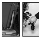
Solution drain hose also functions as the solution level indicator while large recovery drain hose offers soft, squeezable section to enable manual flow control.
