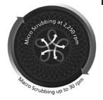
Patented REV random orbital scrubbing technology with high speed 1/4 inch micro scrubbing and 14 inch rotational macro scrubbing attacks dirt from multiple directions for superior cleaning effectiveness.
