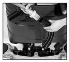
The squeegee hose eliminates the need for a drain hose and also helps rinse the recovery tank clean and reduces dirt build-up.
