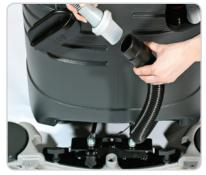
The squeegee hose eliminates the need for a drain hose and also helps rinse the recovery tank clean and reduces dirt build-up.
