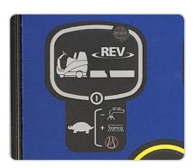
REV<sup>™</sup> Model Only – When in scrub mode, the One-Touch<sup>™</sup> REV<sup>™</sup> function activates floor finish removal operation.
