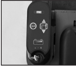
Simple one button control panel.
