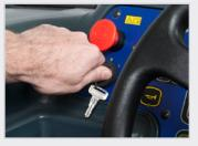
**2** Turn the CS7000 on by turning the ignition key **ON**.
