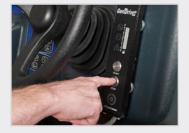
**2** Turn the Fuel Cell off by pushing the **STOP** button.
