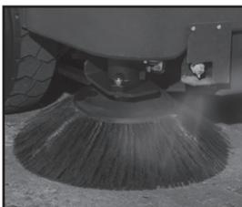
DustGuard™ suppresses airborne fugitive dust where most dust is generated – at the side brooms.
