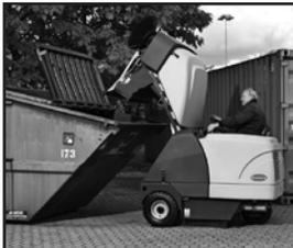
Variable dump height of up to 62 inches allows fast and simple disposal of swept debris.
