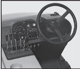
Ergonomic operator interface uses Analog-logic™ which allows a single operator motion to lower and activate the main broom and side brooms and open the hopper door.
