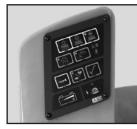
One-Touch<sup>™</sup> activation of scrub system. All systems start and stop with machine motion.
