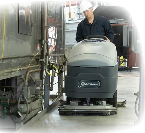
Walk-behind scrubbers are well suited to smaller facilities with a need for scrubbing and light debris pickup.
