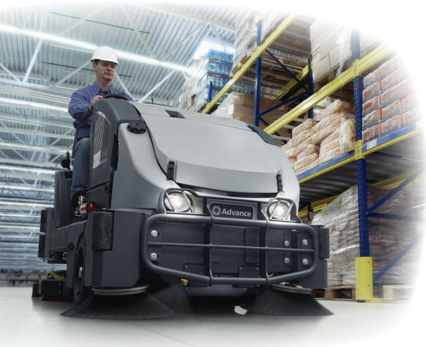
For facilities that require both sweeping and scrubbing, sweeper-scrubbers combine two cleaning functions into one machine.
