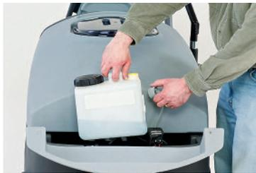
A unique AXP™ dispensing feature on Advance scrubbers and extractors reduces the amount of water and detergent used, eliminates operator exposure to concentrated chemicals, and reduces equipment cleaning and maintenance.
