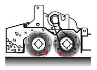
AquaRide sweeper-extractor has dual rotating brushes that sweep and clean both sides of the carpet. A hopper collects the debris.
