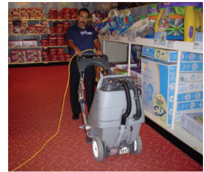
Operators using the Advance AquaClean® 18 FLX can scrub carpets with just the right amount of water, and the dirty solution is vacuumed away in the same cleaning pass.
