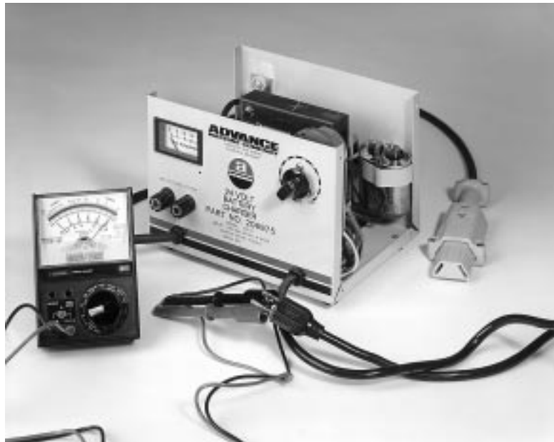
FIGURE 4. Test AC circuit for continuity.
