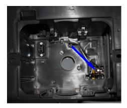
Step 2 Unplug the wires for the Power switch.
